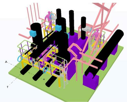
After 2 weeks of design, the steel platform and main support frame, handrail system and GRP floor grating was completed and handed over to the workshop to fabricate.
